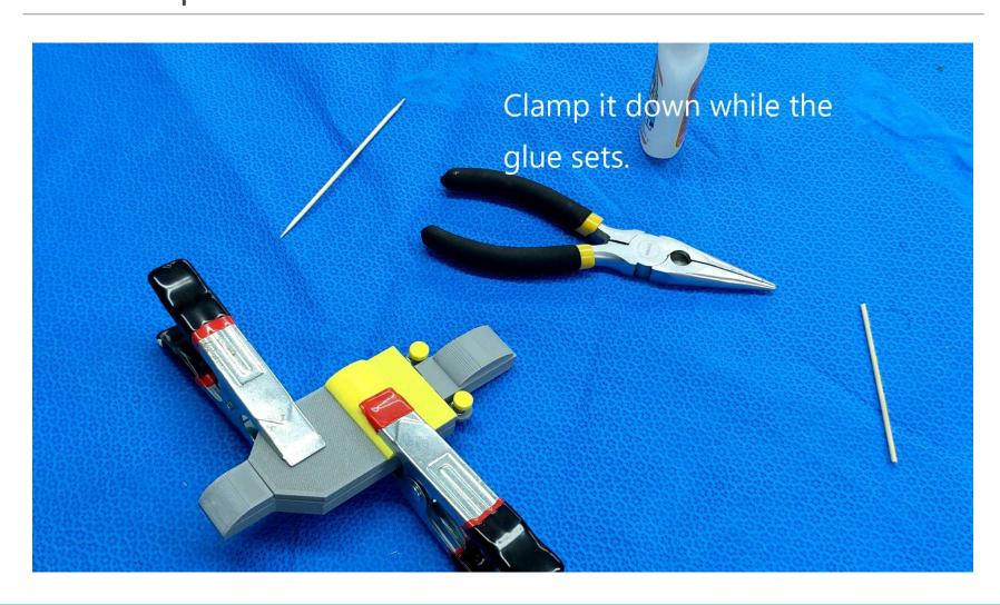
TIP – After clamping, check to be sure the Thumb Rest is aligned properly. Clamping may cause the Thumb Rest to slide out of place.
