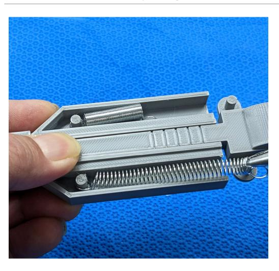
Twist the Spring as you pull to position the End-Loop to lie flat at the bottom of the Spring Post.
