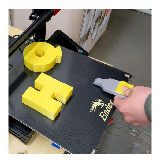
With the Body pressing lightly against your model, release the hammer. The print should come free.
