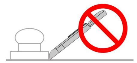
DO NOT ANGLE DOWN TOWARD THE PRINT BED OR DAMAGE MAY OCCUR – SUCH AS SHATTERED GLASS.
