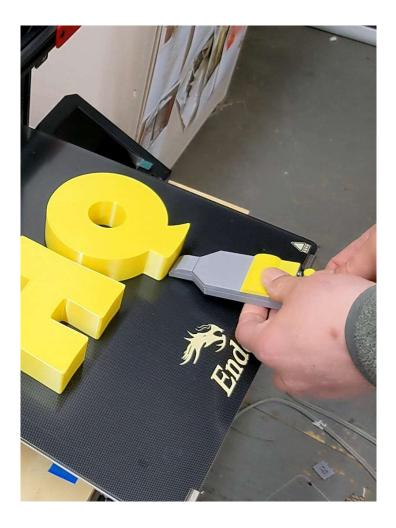
The 3D Print Remover should touch the side of your model lightly, at the bottom against the bed surface.
