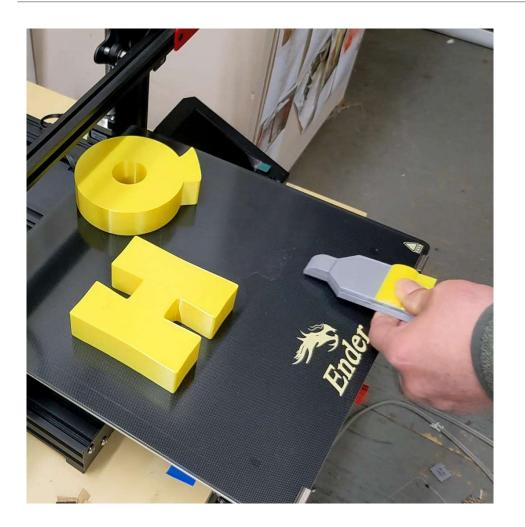
If you have a particularly large 3D print, or the build plate adhesion is quite strong (as with the use of Aqua Net Extra Super Hold Professional hairspray as a binder), it may require multiple "snaps" to remove the print.
