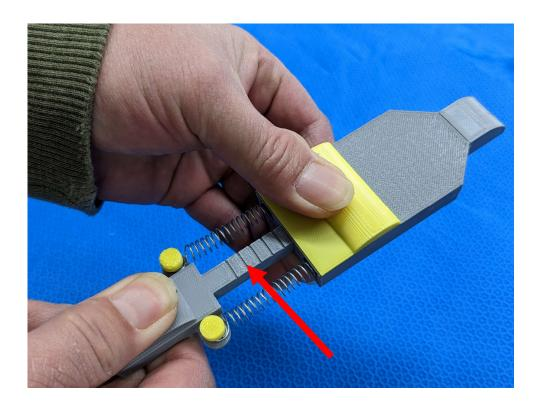
Pull back the Hammer to the second line marking.
